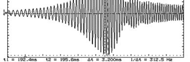
The cursors measured the frequency at the peak of the waveform, and voila the same resonance that we saw in the FFT example. For a little more resolution, I spread the waveform some more, and found the resonance to be at about 333 Hz:
